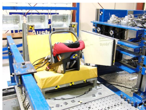
iSize Child Restraint testing with one intrusion cylinder on HyperG catapult
