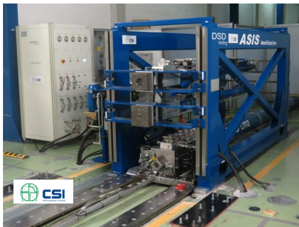
ASIS (Advanced Side Impact) upgrade on floor-integrated catapult
